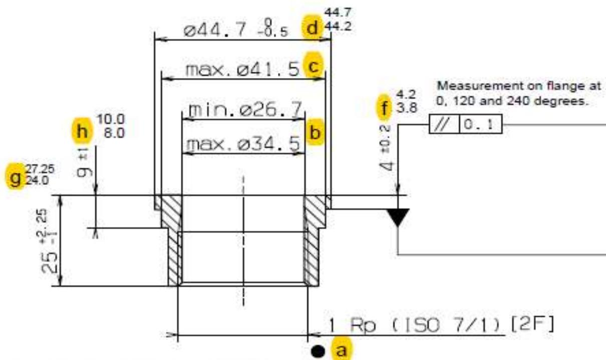
Non stated tolerances according to DIN ISO 2768 MK
